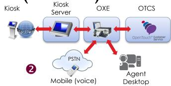
The Kiosk Server application initiates a call between the mobile device and the requested service (routing logic is handled by Contact Center application based on OTCS + data exchange mechanisms)
